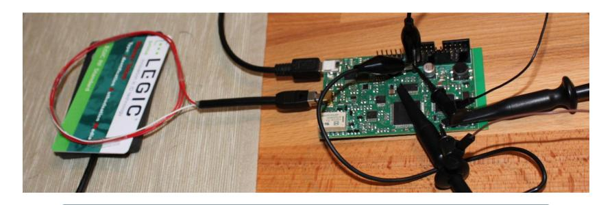
Sniffing with OpenPICC2 (fixed threshold, not so good) or Proxmark3 (hysteresis, much better) and oscilloscope or logic analyzer
