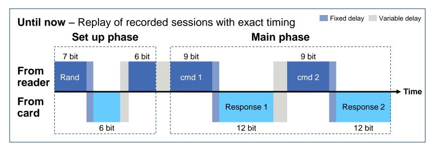
ExperimentVary the timing before the first commandResultCard response for some delays, no card response for othersInterpretationResult of the de-obfuscation changed, which changes the command bitConclusionThe obfuscation stream generator is continuously running (at period time ~100μs)
